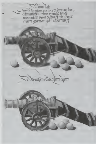
Figure 8: Cast-bronze cannon of Maximilian I of Bavaria. Designed to smash fortress walls with a solid shot of iron, these large artillery pieces were lifted onto their wooden carriages by handles cast into the top of the barrel. Each carriage was carved from a single timber. From Geschützbuch oder Zeugbüch Kaiser Maximilian, about 1500. In the Bayerische Staatsbibliothek, Munich (Cod. icon. 222, fol. 45v). Bayerische Staatsbibliothek, Munich
